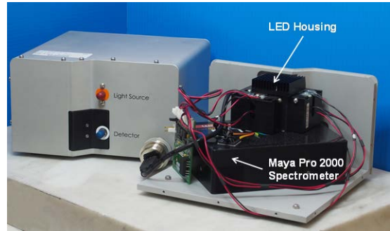
Figure 2: Custom-made fluorometer with internal components
