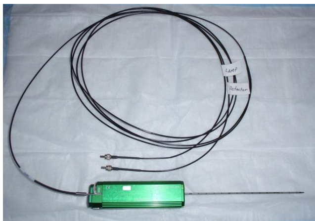
Figure 1: Optical biopsy needle with BARD Urological MAGNUM biopsy gun
